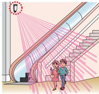
Mount up to 6m in height with a coverage of 49' (15m) x 80° 'high density mode', perfect for high installations such as open ceiling entrances.
